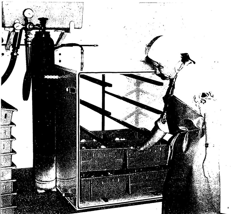
Figure 1 Chamber and apparatus for carbon monoxide euthanasia.
