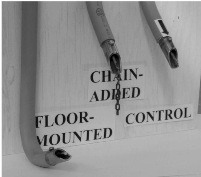
**Fig. 1.** From left to right, the floor-mounted, chain-added and control nipples. A continuous drip adjustment screw was installed on all nipples to allow the continuous drip feature to be used as required (arrow on 'CONTROL' nozzle shows screw location).
